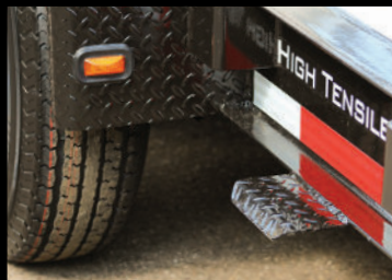
Step To Access Deck
