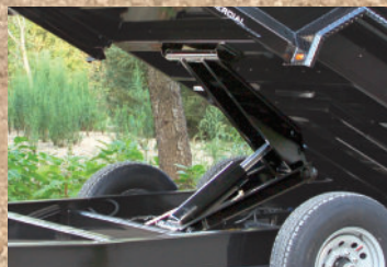
Scissors Hoist Standard on 12' & 14' (cylinder on 10')
