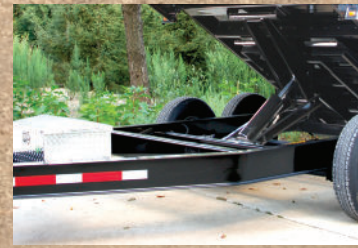
8" I Beam Frame
