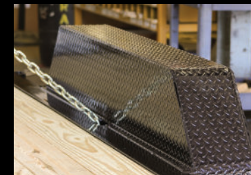
Tie Down Between Fenders (flush w/deck & fenders)
