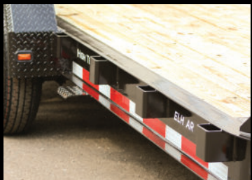
Heavy Duty 4" x 1/4" Bar Stake Pockets
