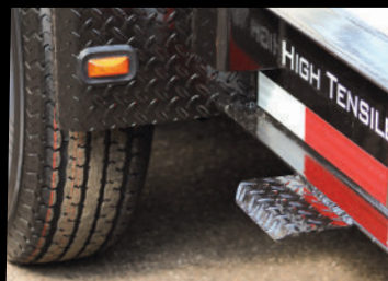
Step To Access Deck
